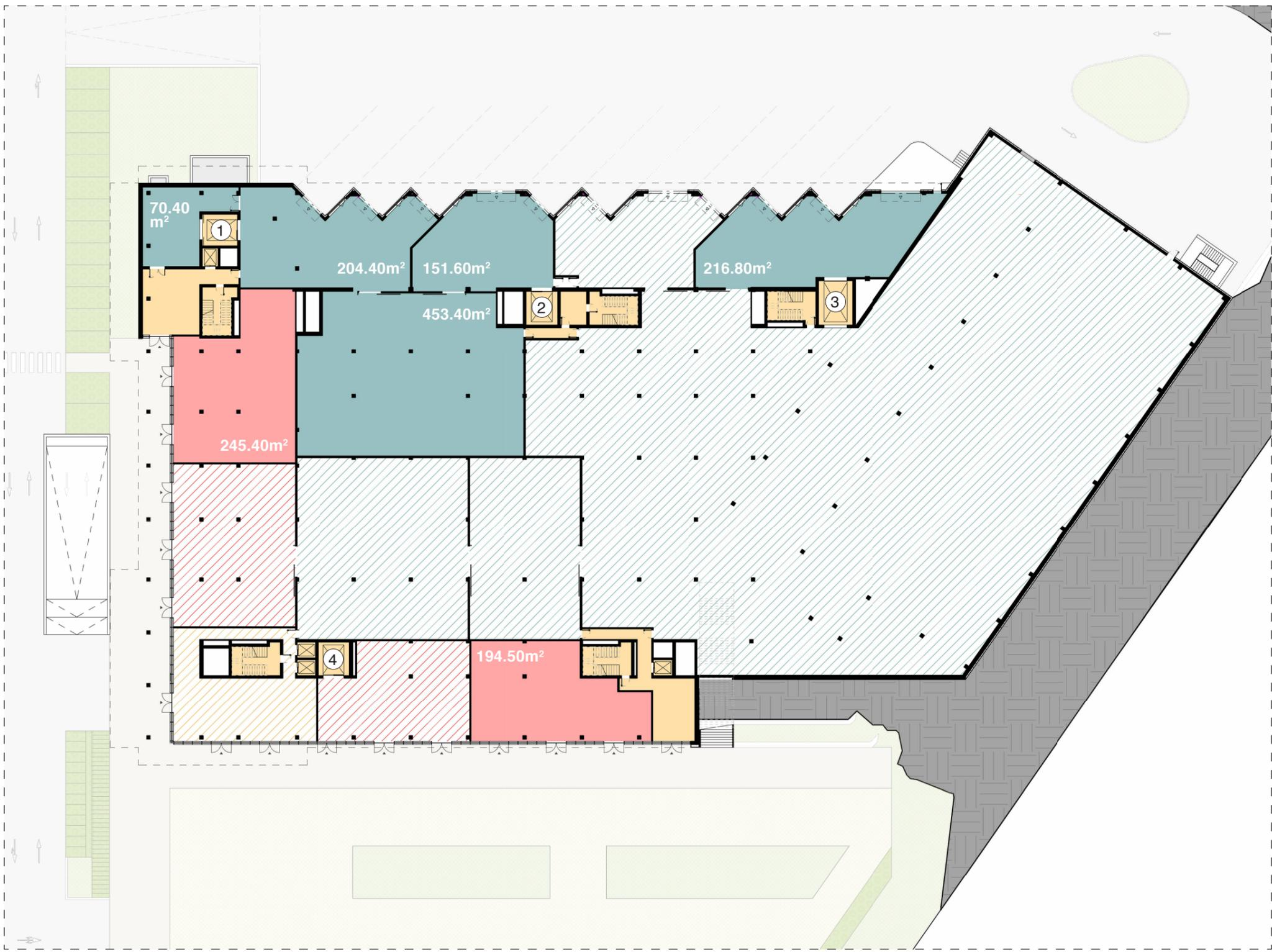
① MCharge A - 4T - H300    ② MCharge B - 4T - H220    ③ MCharge C - 6T - H240    ④ MCharge D - 4T - H220
